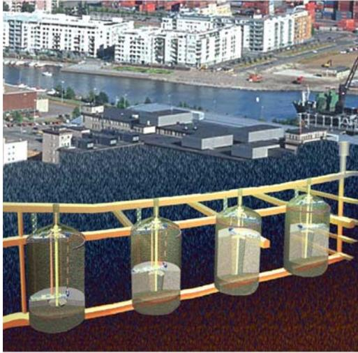
Fig. 6. Underground Eurosilos coal storage at Salmisaari Power Plant
