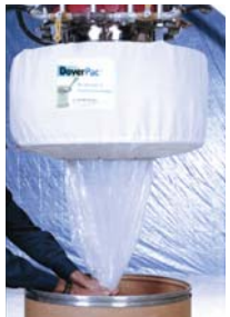
Sleeve is pulled into drum and filled
