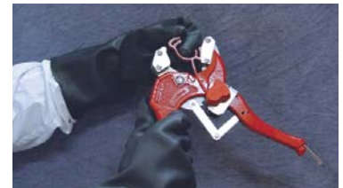
Load crimp into installation tool
