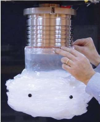
Attach neck of continuous liner to canister
