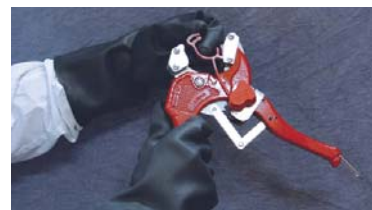
Load crimp into installation tool
