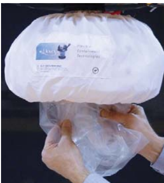
Pull down liner material to start processing
